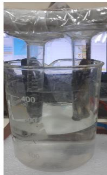
FIG. 3: Illustrates lab-made simple electrolyzer for salty groundwater;
