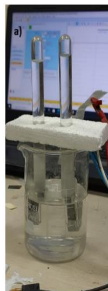
FIG. 2: Illustrates lab-made simple electrolyzer in KOH treated seawater and production of O 2 and H 2 collected in inverted glass tube;
