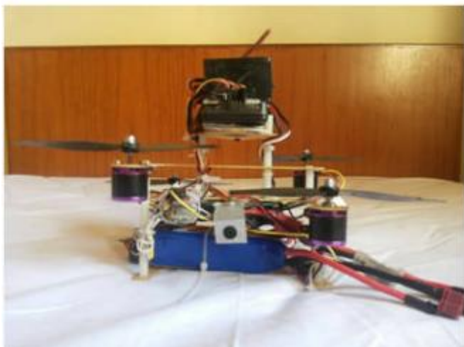
Fig. 3a: Illustrates prototype of the VOOPS Quadrotor configuration in landed mode
