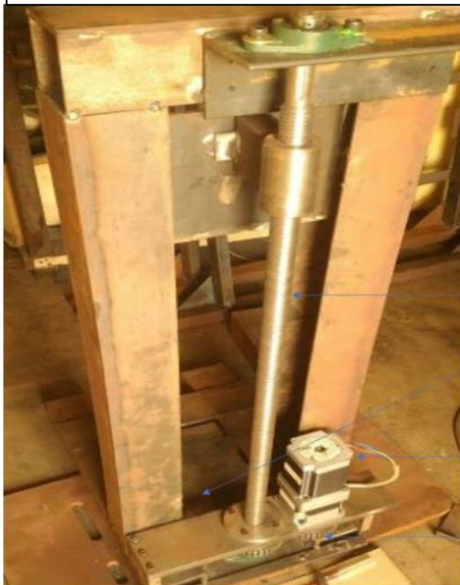
Fig. 3. A lifting mechanism using lead screw and motor
