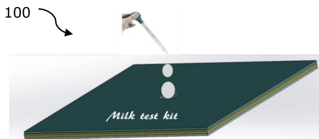
Fig.1: Illustrates a schematic view of the 3D paper-based microfluidic device for detecting multiple adulterants in liquid foods and beverages.
