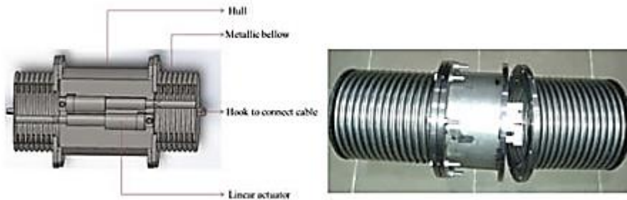
Fig. 2 depicts double bellow variable buoyancy system.
