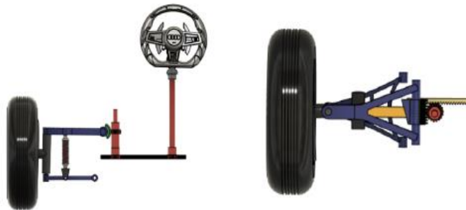
FIG. 3A. illustrate a front view and a top view of the camber adjustment mechanism depicting wheels in a neutral position.
