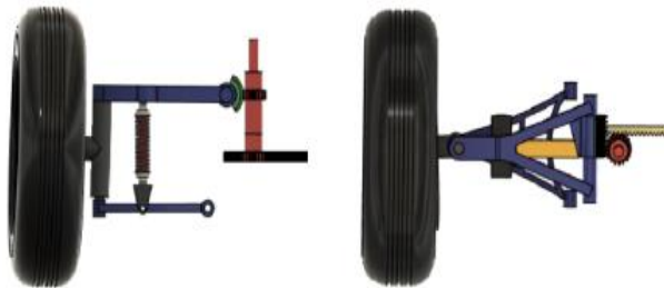
FIG. 3C. illustrate a front view and a top view of the camber adjustment mechanism depicting wheels in a negative camber configuration.
