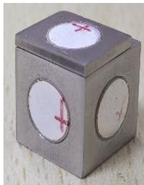
FIG. 1 depicts an ME based press-fit magnetic sensor, in accordance with an embodiment;
