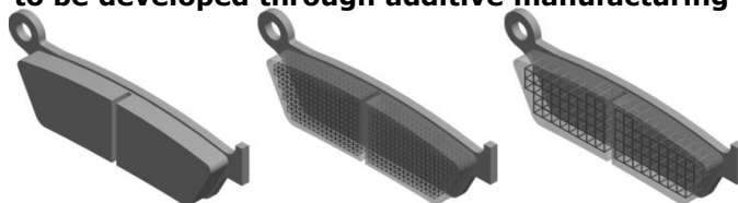
Figs. 2 shows 3D models of a brake pad required to be developed through additive manufacturing
