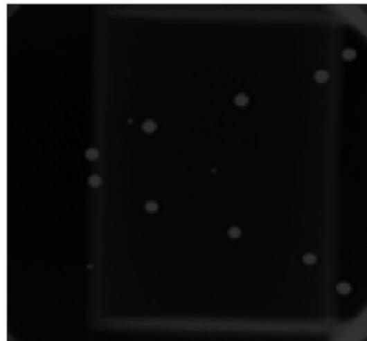
**FIG.4A.** illustrates shots appearing as 2D projections of the spiral object when taken at roughly equi-spaced poses with this object placed stationary under the c-arm.
