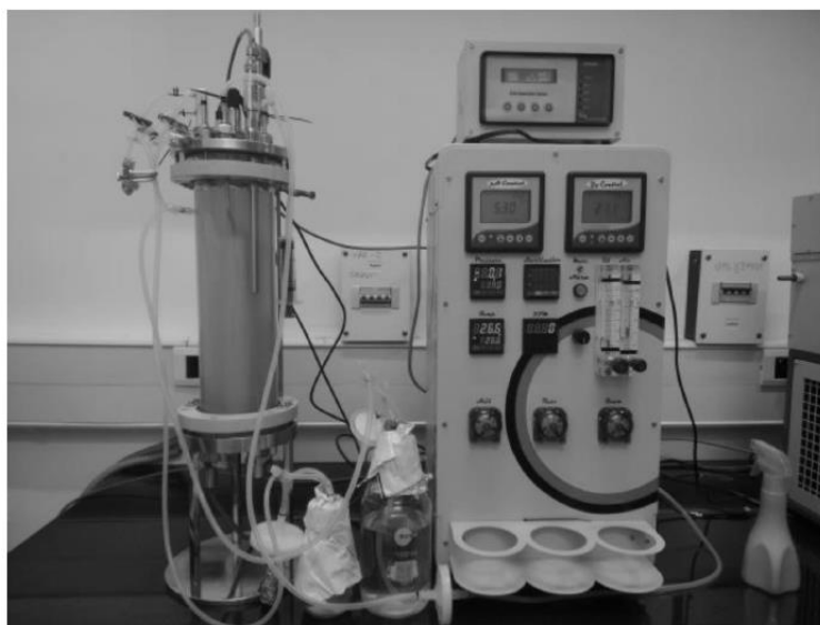
FIG. 2. Airlift reactor (ALR) for biomass production of Viola odorata L.
