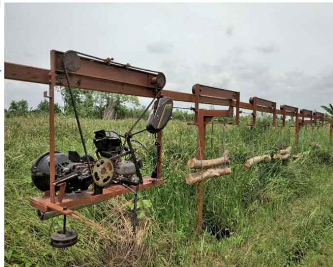
FIG.1 shows the photograph of the upright steel posts and lightweight steel rails erected along the edge of a farm with the traction trolleys and the loaded trolleys
