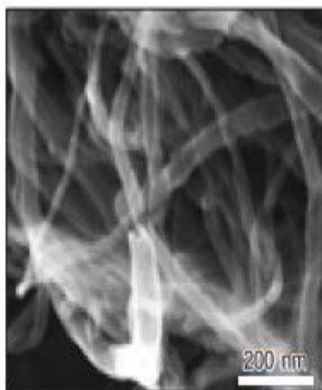
FIG. 2B shows the EDX image of S@PCNT that confirms the incorporation of sulphur in the unzipped randomly oriented carbon nanotubes
