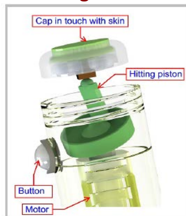
Fig 1. illustrates the motor with the eccentric plate and piston.
