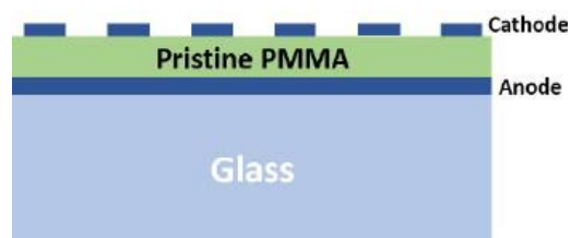
Fabricated PMMA based Metal-Insulator-Metal (MIM) devices
