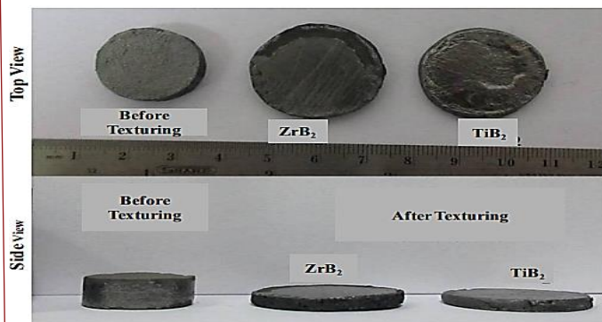
FIG. 3 illustrates the compacts of TiB 2 & ZrB 2 before & after texturing.
