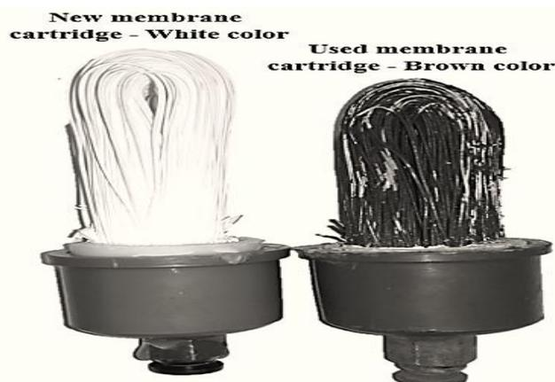
FIG.2: Illustrates the change in cartridge colour with use
