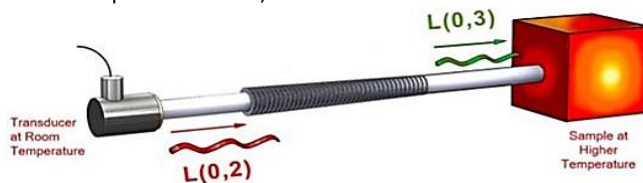
Fig.2 shows the use of proposed MeTradd filter with tapered baffles illustrating that the selective generation of enhanced L(0,3) mode in the rod leads to the effective generation of bulk longitudinal waves in a target sample at a higher temperature.
