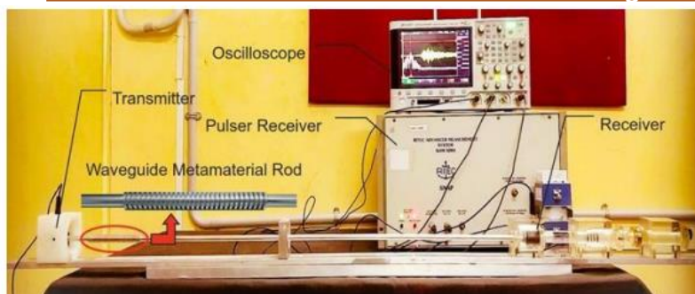
FIG.4: Illustrates an experimental setup showing the MM rod clamped between the transducers with the help of spring-loaded mechanism;
