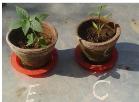
Figure: The biodegradable super water absorbent polymeric material made from chitosan, citric acid and urea (CHCAUR-labeled E) appears to be doing far better than the control (labeled C).
