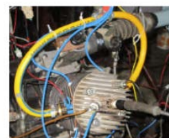
FIG. 1. Depicts the test set up and cylinder barrel with injectors of the injection system showing injectors (1a).
