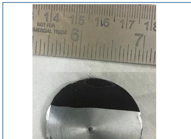
Figure: Photograph showing the polished part of a specimen and the part subjected to patination upon exposure to the alternative chemical solution.
