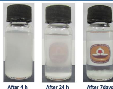
Figure: Photographs showing the flocculation of NCC dispersion with time
