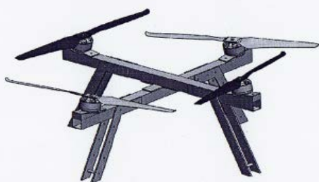
Fig 3. VOOPS with inclined mounted motors
