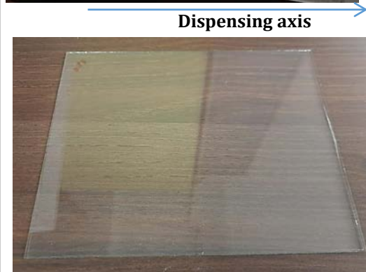
Fig 7: Output after cover-slipping - no air bubbles
