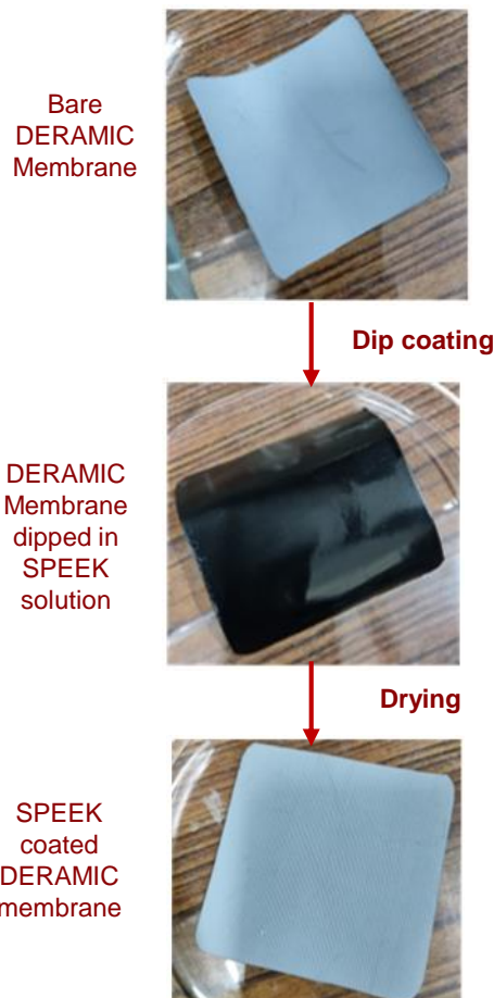
Figure: Preparation method of DARAMIC/SPEEK membrane
