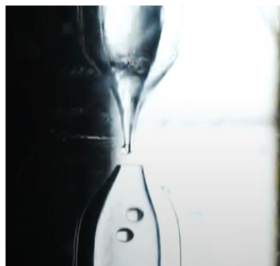
Figure: Photograph of micro-droplet generation at the microfluidic junction of the microfluidic device.
