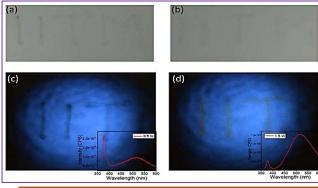
Optical emission PL spectra of ZnO nanoparticles prepared with range of different pulse-widths and ablation power.
