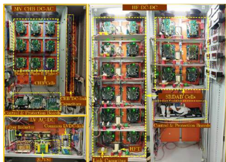
Figure: The Hardware Prototype- The proposed control is verified on a developed 1.2kV(MVAC)/400V(LVDC)/200V(LVAC), 20kW CHB-based PET prototype setup. The entire control architecture is implemented on a DSP and FPGA-based hybrid control board..
