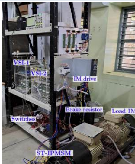
Figure: The proposed concepts have been validated on a 3.7kW IPMSM setup.
