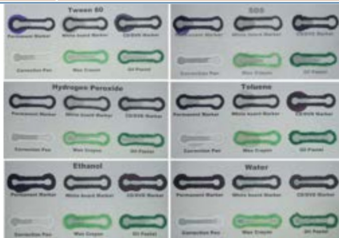
Figure: Chemical retaining ability of different material sketched channels on Grade 1 Whatman(R) cellulose filter paper with 1 min heating at low flame (n=3). The figure demonstrates the superior chemical retention capability of oil pastel barriers compared to conventional alternatives.
